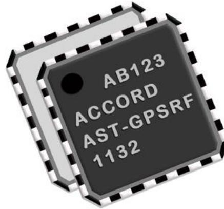
AST-GPSRF is a high performance, fully integrated GPS / Galileo RF front-end chip for down conversion and signal amplification. It is designed for GPS L1 (1575.42MHz), C/A and Galileo OS (1575.42MHz) receivers. It can also process the signals from SBAS satellites.
