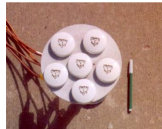
Figure 2: Antenna array assembly.
